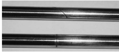
Fig. 9. Transverse-cracked shaft and 45° slant-cracked shaft.
